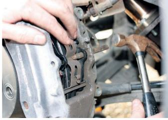
bolts you reuse rather than replace will require some anti-seize grease to ensure they don't get stuck in future. The new pads will want some copper grease on the back of them, so too the anti-vibration dampers that sit behind them, the pads can be lubricated down their sides too where contact will be made – ensure you don't get any on the face of the pad though. With everything back together, including the fitment of fresh wear sensors, top up your brake fluid reservoir with
